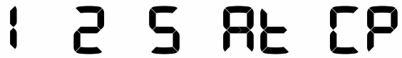
1 Target Tone 2 Target Tones 5 Target Tones All Tones (At) Continuous Pitch (CP)
