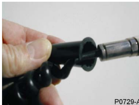
Figure 15: Removing Coil Plug Retainer
