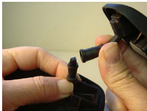
Figure 29: Connecting Speaker Pod to Wiring Loom
