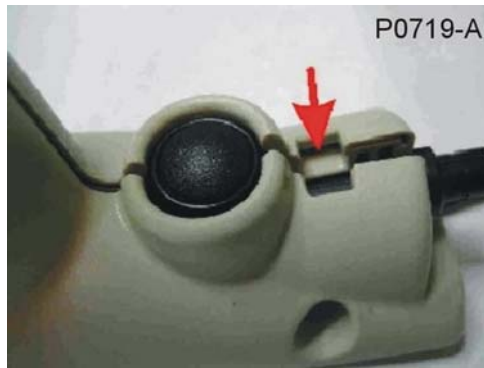
Figure 33: Recess for Earset Plug Dustcap
