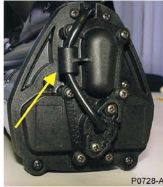
Figure 41: Wiring Loom Routing
