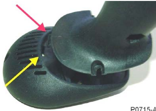
Figure 27: Fitting Speaker Pod onto Handle
