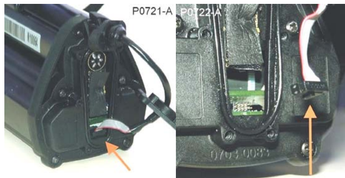
Figure 35: Removal of Wiring Loom from Electronics Pack
