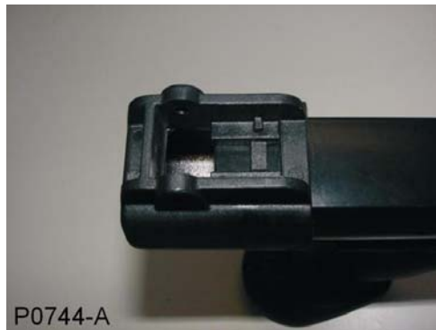
Figure 48: Upper Camlock Positioned on Upper Shaft
