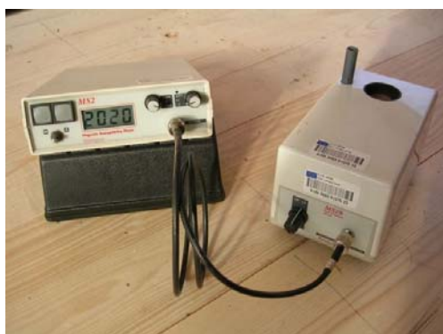
Plate 6-2 Bartington MS2 configuration for sample (MS2B-left) and field measurements (MS2D-right)
