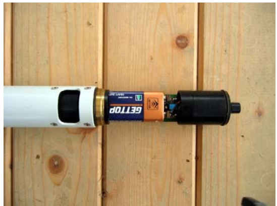
From left: sensitivity adjustment, battery compartment, internal speaker and power knob.
