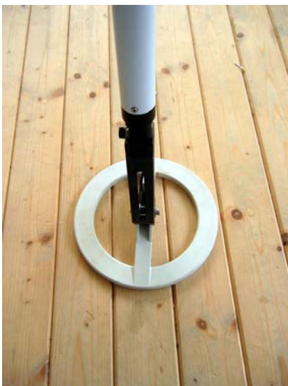
The detector in short configuration with the rechargeable battery pack The armrest and handle are not displayed
