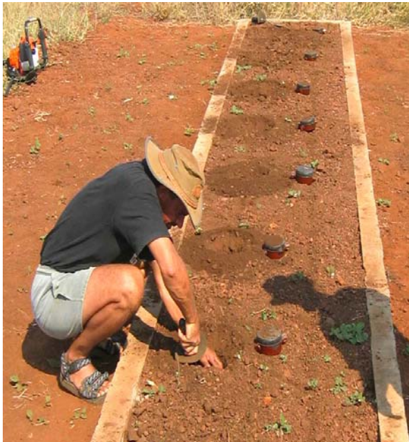
Plate 5-5 Burial of the PMN mine – because of its large detection halo, only one line was used
