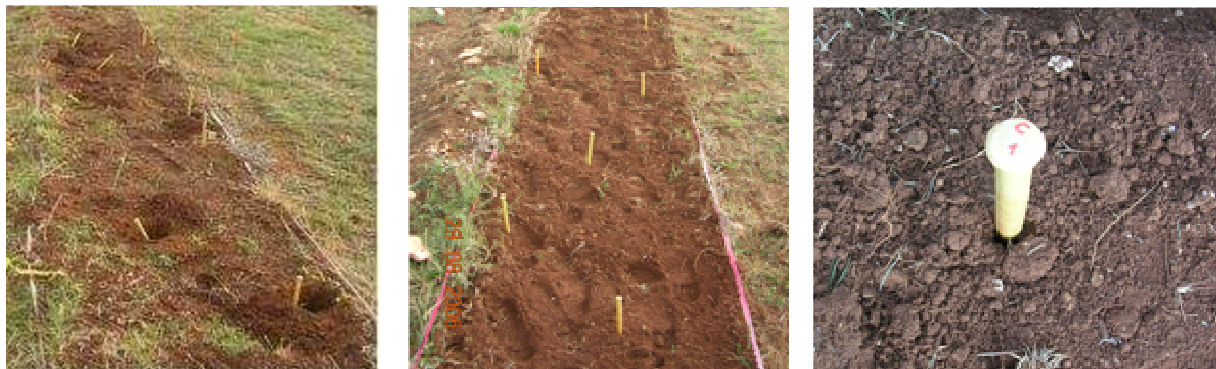
Figure 5: Different stages of lane preparation – a) depth, b) buried, c) used for position & depth measurements
